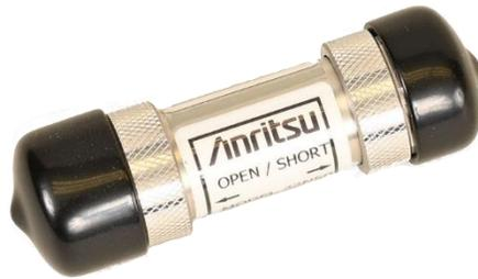
**Figure 2-10 VSWR Open/Short Calibration Load**
